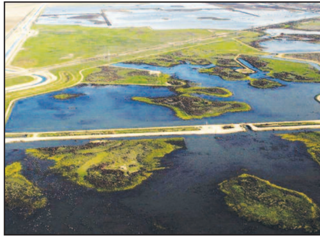
The Kern Water Bank in southwest Bakersfield, California, has 20,000 acres of groundwater recharge basins. Kern County Water Agency
